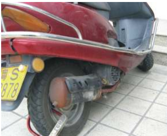
CORROSION OF MUFFLER OBSERVED
