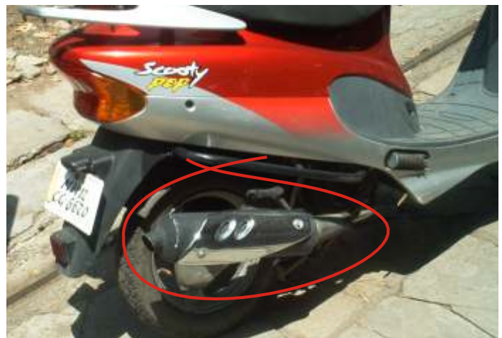
AFTER 5000 KMS RUNNING, ABSENCE OF CORROSION OR CHALKING MUFFLER IS COATED WITH ORBIT HR POWDER
