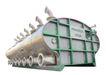
The purpose of de-inking is to remove the printing inks and other substances like stickies that might effect the paper making process or the final properties of the paper. In a de-inking process the ink should be first detached from the fiber. Flotation technology with high efficiency provides high yield of fibers and simple handling with maximum operating reliability.
