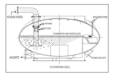
Flotation process operated a continuous mode and helps to remove ink particles efficiently. Since the cells are interconnected by opening only level control system is required for entire flotation machine.
