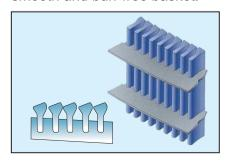
Flow in profile edge creates more turbulance, improving throughput and cleaning efficiency.
