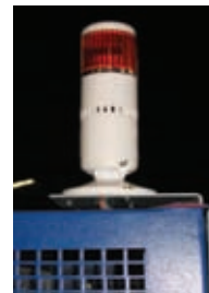
Tower lamp with buzzer for no tape alert
