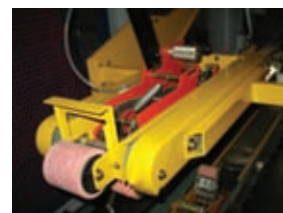
Belt guards-operator safety
