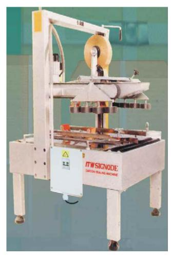
ITW Signode's 4AM/6AM Carton Sealing machines are manufactured for reliability and efficiency. Recommended for applications where the same sized cartons are sealed consequently. Designed for throughputs ranging from 10-40 cartons/min. depending on the size of the carton.
