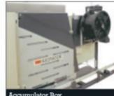
The accumulator box is used to temporarily store the strap between the dispenser and strapping head before it is fed through the chute system, thereby optimising the feeding performance.
