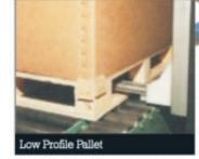
Strap is fed via a torque-motor driven bayonet through the pallet void.
