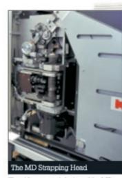
The side-mounted design of the MD strapping head enables it to securely strap pallet loads of differing widths without any loss of tension. The pallet side is detected via a sensor and the MD head moves towards the pack at the optimum approach speed to prevent any damage to the pallet. The MD head requires only minimal maintenance and consumable parts.
