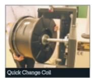
The quick-change coil dispenser allows strap coils to be changed without delay.
