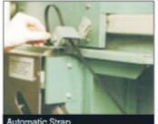
All Signode MD machines are equipped with a fully automatic, highspeed strap feed system to maximise machine availability.
