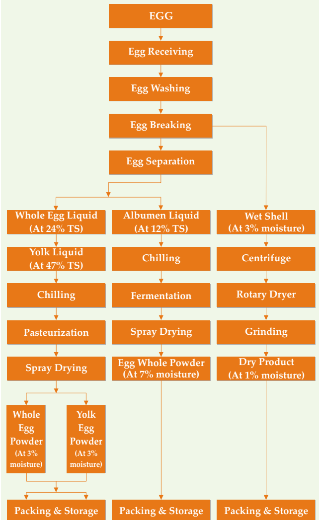
FLOW DIAGRAM FOR EGG PROCESSING PLANT
