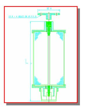
Vidyut range of breathers provide an economic and efficient means of controlling the level of moisture entering electrical equipment during the change in volume of the cooling medium and/or airspace caused by temperature gradients.
