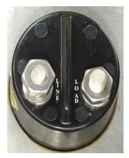
Feed the positive up through the remaining hole, which should be the hole closest to the tail-gate. Attach the red power to the power terminal marked "Line" on the On/Off Switch. Run the ground line from where it is secured on the lift frame run it down through the same hole and mount it to the chassis under the truck. Insure that the terminal attaching points are clean to bare metal. Connect the Power Cord to the truck's battery terminal.
