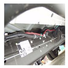
Run the long Power Cord under the truck bed and attach it to the chassis with the supplied tie wraps. Pass the power cord end through the hole in the bottom of the pump compartment of the Unit Frame.
