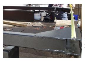
Next, with the unit positioned, measure the distance from the outer edge of the front arms to the outer edge of the front arm. The distance should be 85 1/2" within an inch.
