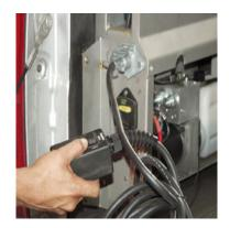
Plug the female fitting into the receptacle on the rear of the pump side frame. Depress and hold the "Boom Out" button.
