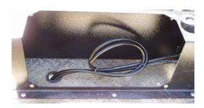
Once the hose ends are connected to the pump pull the excess hose lengths out of the Pump Housing and bring the slack back to the space in the Unit Frame on the passenger side. Use the tie wraps and secure the hoses to the chassis under the truck, coil the remaining length in the passenger side space and use the tie wraps to hold the coil together.
