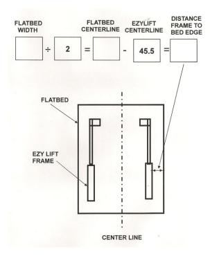
Place the two Unit Arm Frames on the flat bed. The frame without the Hydraulic Pump is on the passenger side of the flat bed.
