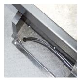
Take the hose ends found in the space on the passenger side's frame space and pass them down through the hole. Set the hose ends aside.
