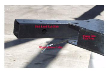
Locate the Winch Power Cable in the pump side arm and pull the ends out of the arm. Connect the power cable to the fish lead and pull the fish lead through the Winch Power Cable Feed Hole. Set the electrical leads aside.
