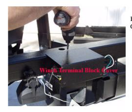
Back out the three screws that secure the Winch Terminal Block Cover. Remove the cover and set it aside.
