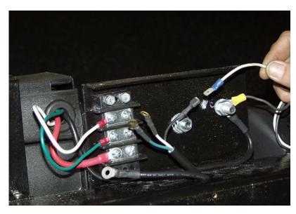
Connect the Winch Power Cable leads to the winch terminal block. The black lead connects to the red lead. Connect the green lead to green, the white to white and finally, the blade connection to the blade receptacle.
