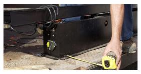
Use the number, (Distance Frame to Bed Edge), arrived at in the equation above and the tape measure and adjust the position of the Unit Arm Frames so that they are exactly parallel with the edge of the bed and exactly the distance from the bed edge the entire length of the frames. With the permanent marker mark the bed through the outside rear frame mounting hole and the inside front frame mounting hole.
