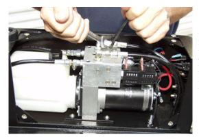
Bring the hydraulic hose ends up through the hole in the Pump Housing to be connected. Remove one of the fitting-plug from one of the hoses, affix the end to the valve fitting and tighten. Repeat with the other hose end. The larger (#6) fitting requires an 11/16" wrench and the smaller (#4) requires a 9/16" wrench.
