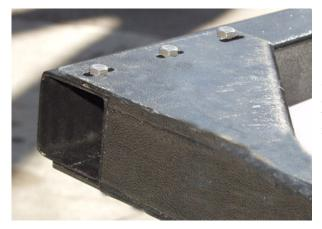
Secure the crossbar to the unit arm brackets with the 5/16" x 4" bolts and the lock nuts. The crossbar fit into the bracket is extremely tight. It may be necessary to tap it in place with the rubber mallet.
