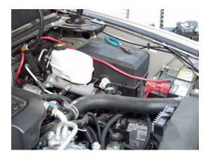
short Power Cord. Position the short cord from the battery to a clear area of the truck's engine compartment firewall. Mount the Fuse Box to the firewall in this area. Connect the short cord to the Fuse Terminal closest to the battery. Pass the end of the long up into the engine compartment and connect it to the other Fuse Terminal. Place the Fuse Box cover on the Fuse Box and secure.
