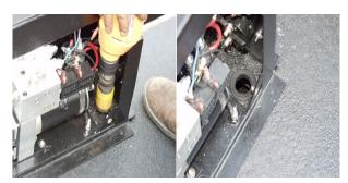
Use the drill and 1" Hole Saw Bit and drill the cord and hose hole where the center point is marked. Once the hole has been drilled use the rasp to smooth the edges and insert the rubber grommet. After these steps, reposition the Unit Frame by aligning the two holes previously drilled with the Unit Frame mounting holes and reinsert the screws attaching with the washers and nuts. This time tighten these screws securely.
