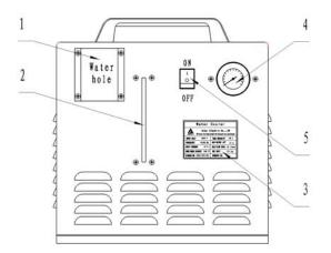
Figure 14: Front panel of water cooler
