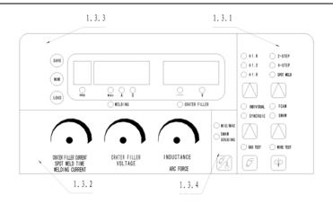
Figure 7: Welding machine control panel
