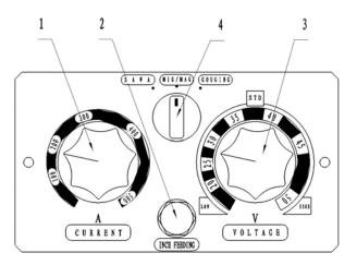
Figure 13: Panel of controller
