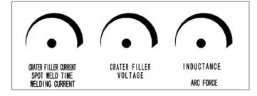
Figure 9: Parameters setting knob
