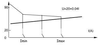
Figure 3: CC Volt-Ampere curve
