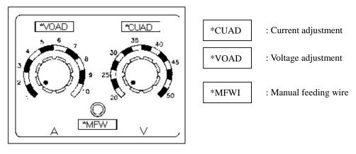
(Picture 5) Controller panel diagram
