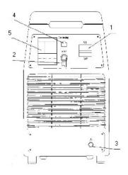
(Picture4) Back panel of welding machine
