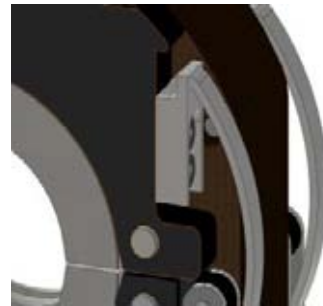
Adjustable spring-loaded system: to account for tube "out of round"
