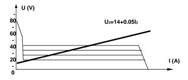
Figure 2: MIG Series Volt-Ampere Curve
