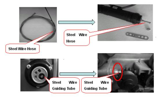
Figure 13: Installation guide for steel wire hose
