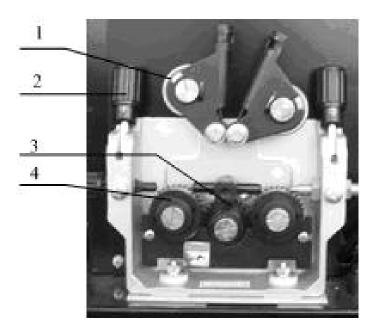
Figure 11: Wire Feeder Structure
