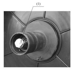
Figure 15: Brake Force Control Screw
