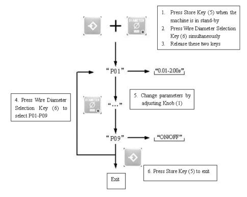
Figure 7: Sub-Menu Parameters Regulation Guide
