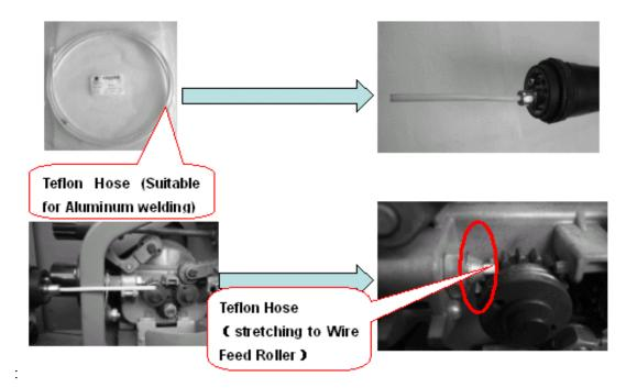
Figure14: Installation guide for Teflon wire hose
