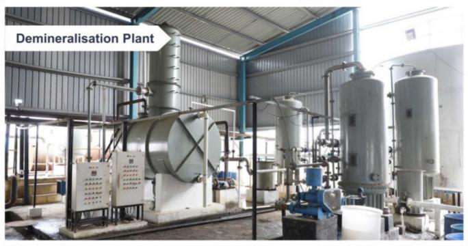
Demineralization is the process of removing mineral salts from water by using the ion exchange process. The DM plant comprises of strong acid cation, strong base anion & mixed bed unit. This results in less than 15 micro Siemen/cm conductivity.
