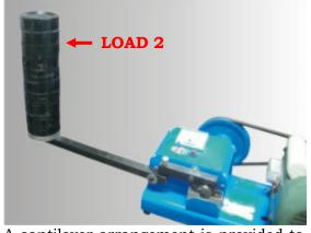
A cantilever arrangement is provided to hold and apply load on the steel billet.
